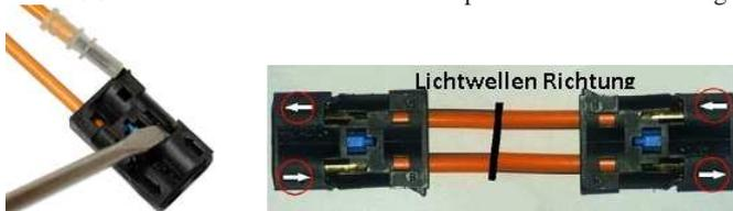
2. Exempt fiber optic cable with Trioma inner plug connect (light direction - in) > the interface. Fiber optic cable with plug - 1 piece (supplied)
