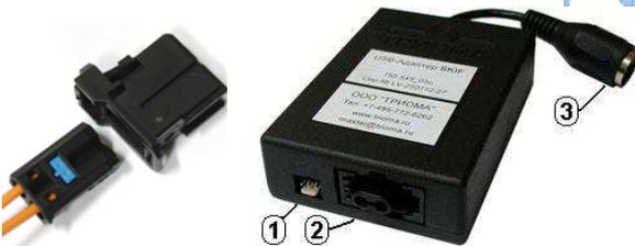
4. Free existing fiber optic cable <connect with MOST connector from the CD changer (in the trioma interface (out))>
