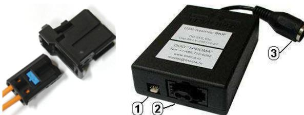
4. Free end of the existing fiber optic cable from the Trioma-Interface (out <) with MOST connector from CD changer to connect (in >)
